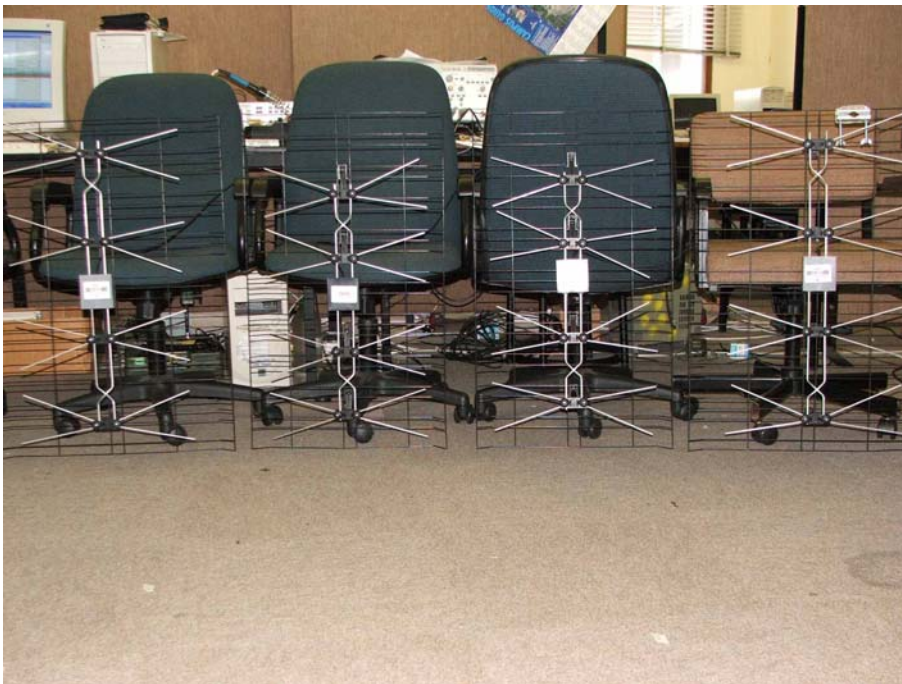
Figure 6.22: Ellies grid antenna configuration for the three channel setup
