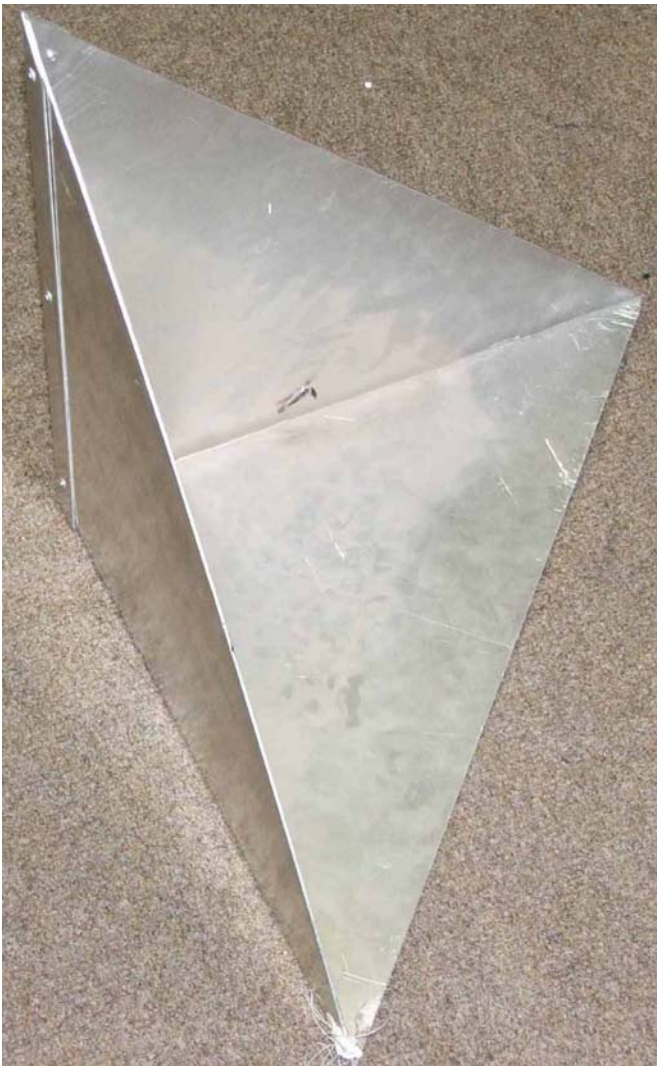
Figure 6.14: Pyramidal corner reflector used as target/reflector
