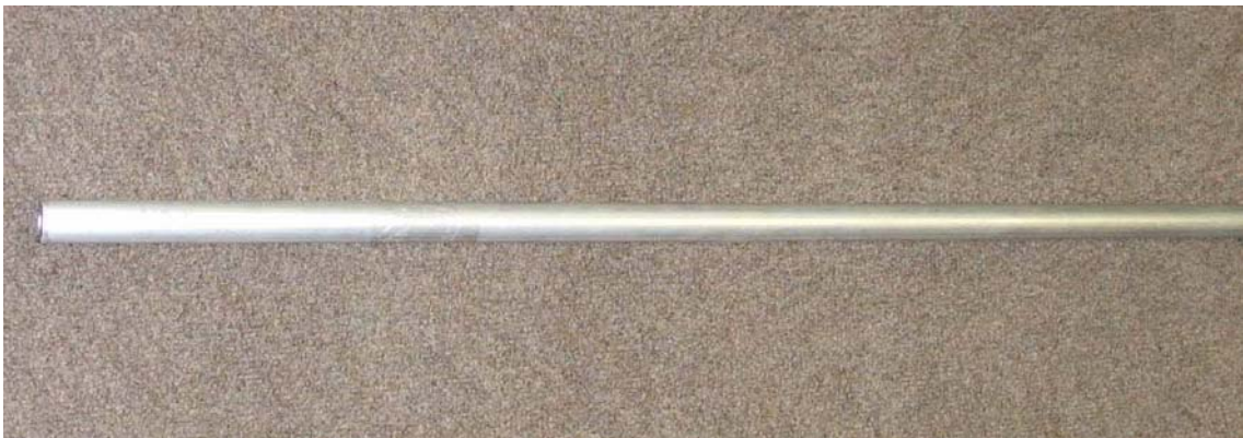
Figure 6.12: Metal pole used as reflector/target
