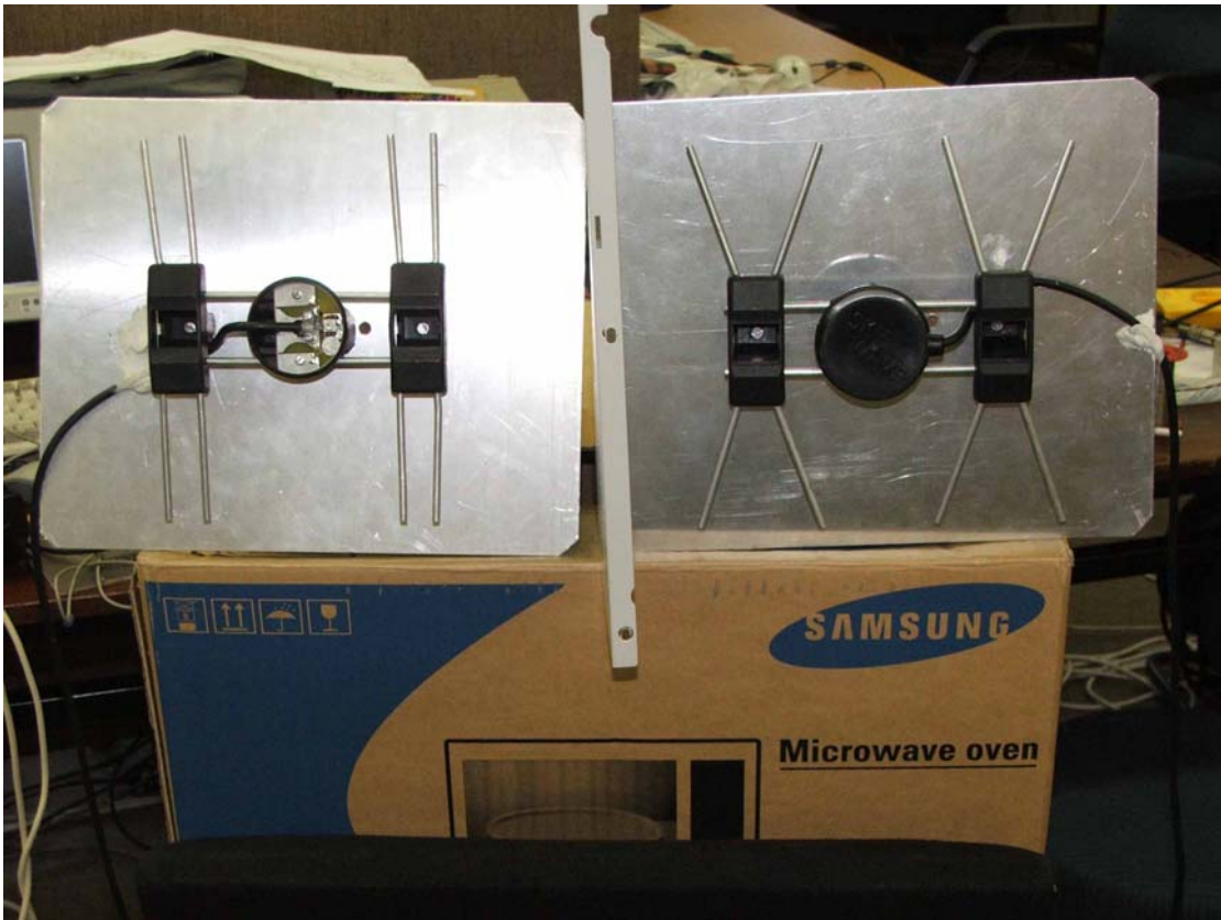
Figure 6.11: Twin bow-tie antenna configuration for single channel testing
